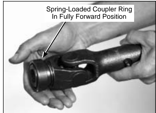
Coupler Ring "Locked" Position
